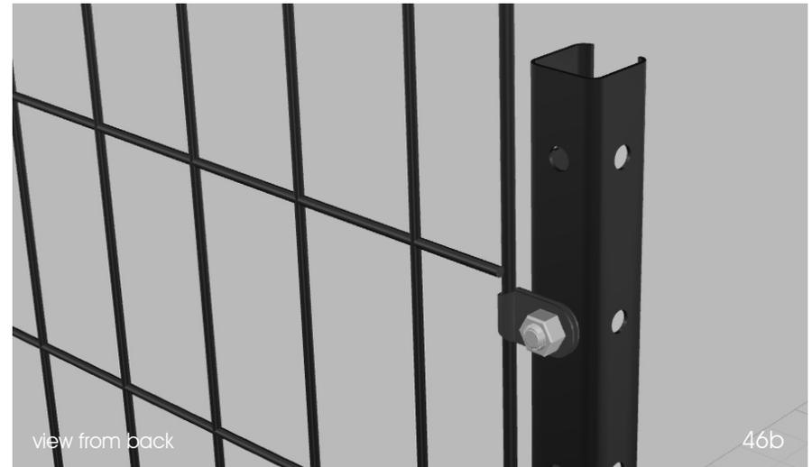
14. Fasten the other three connector washers on the steel wire panel to extension poles with bolts and nuts, as shown in Pic.47.
