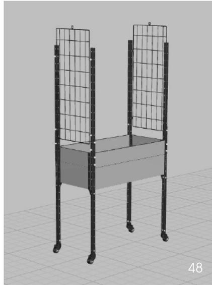
15. Install another steel wire panel follow step 8 to 12, as shown in Pic.48.
